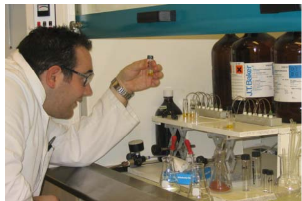
Evaporation of sediment samples in preparation for hydrocarbon analysis
